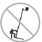
Do not operate the machine in strong or gusty winds. Increasing the load surface area will decrease machine stability in windy conditions.
