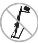
Do not raise the load unless the machine is on a firm, level surface.
