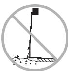
Prior to use, check the work area for drop-offs, holes, bumps, debris, unstable or slippery surfaces or other possible hazardous conditions.
