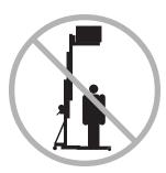
Do not stand under the load. The safety brake system (if equipped) will allow the load to drop 1 to 3 feet / 30 to 91 cm before locking the columns.
